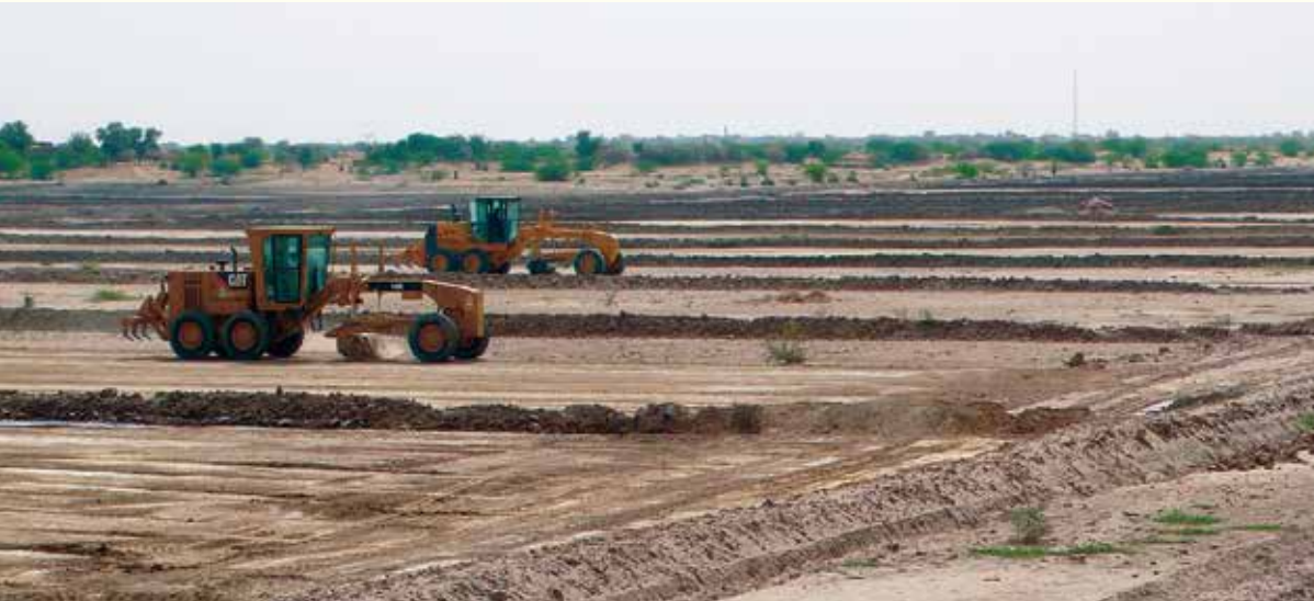
平地机正在对1200公顷范围内农田进行精确平整 Motor graders are used to leveling the 1,200 ha farmlands
